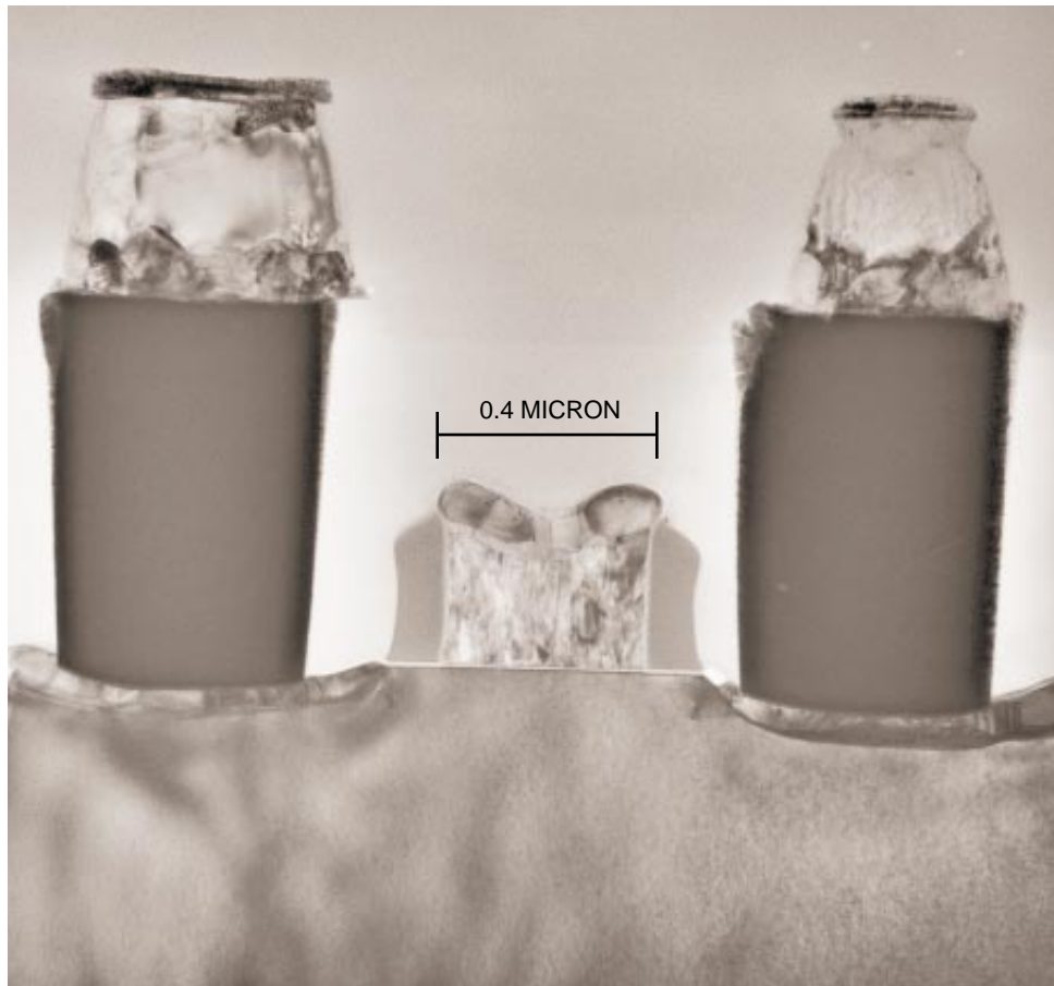
above, left). A contemporary transistor, shown in profile through a transmission electron microscope (right), measures about two microns across and has elements as small as 0.4 micron.
