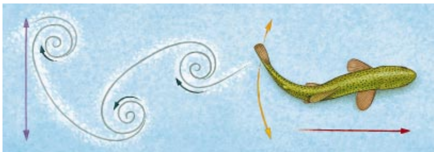
FISH OF ALL KINDS flap their tails to create vortices that produce a jet of high propulsive efficiency. Key parameters describing the jet are related in a ratio known as the Strouhal number, defined as the product of the frequency of tail flapping (yellow arrows) times the jet's width (purple), divided by the fish's speed (red). A Strouhal number between 0.25 and 0.35 is a hallmark of efficient swimming.
