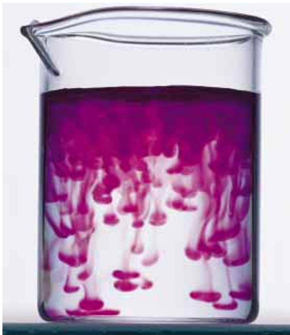
PURPLE FINGERS develop when warm, saline water containing potassium permanganate (which acts as dissolved salt and colorful tracer) floats on cold freshwater.
