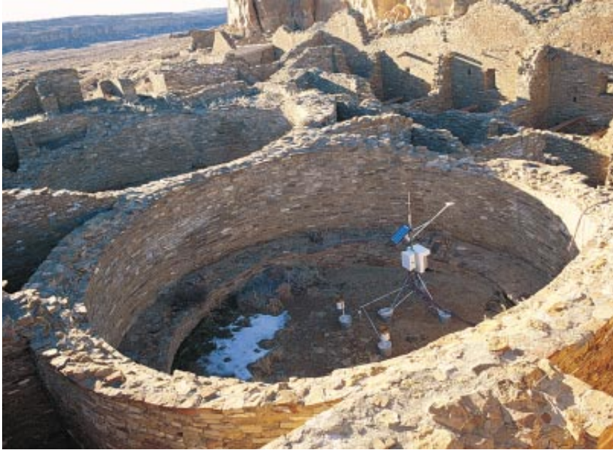
MONITORING STATION sits in a kiva at Chetro Kettle. The device, designed by the Getty Conservation Institute, records changes in soil temperature and moisture. The data may help researchers determine how best to rebury ruins.
