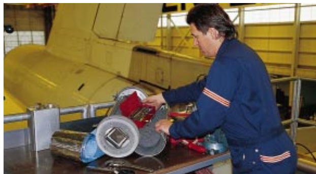
AIRBORNE EXPRESS by pneumatic tube delivers tools and repair parts at the Denver International Airport.
