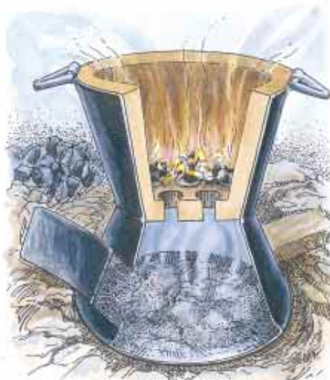
KENYA CERAMIC JIKO (left) increases stove efficiency by addition of a ceramic insulating liner (the brown element), which enables 25 to 40 percent of the heat to be delivered to the pot. From 20 to 40 percent of the heat is absorbed by the stove walls or else escapes to the environment. In addition, 10 to 30 percent gets lost as flue gases, such as carbon dioxide.
