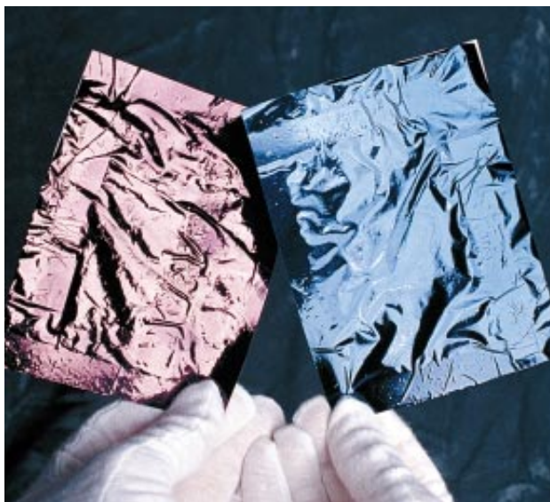
POLYMER SHEETS made of polyaniline appear as a lustrous pink (left) until doped with iodine, which makes the substance conduct and colors it blue (right). Weigong Zheng of the University of Pennsylvania prepared the material.
