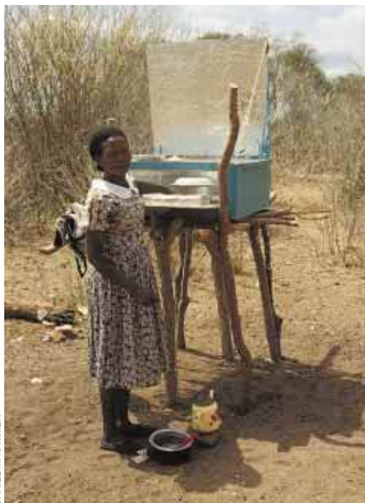
SOLAR OVEN , shown in Kenya, cooks food in a glass-covered box where pots are placed.
