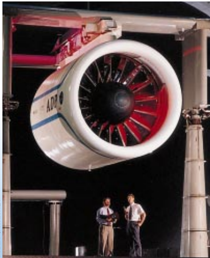
A high-bypass jet engine, such as this one being tested by Pratt & Whitney, will provide greater thrust to power large aircraft.
