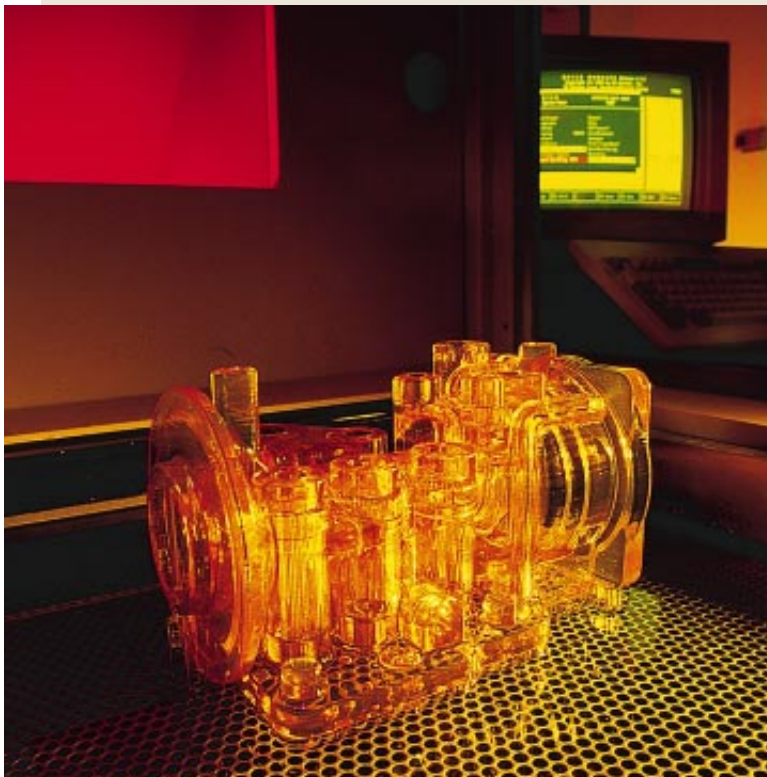
OIL PUMP MODEL was built with stereolithography, a technique for building up structures layer by layer with a laser.
