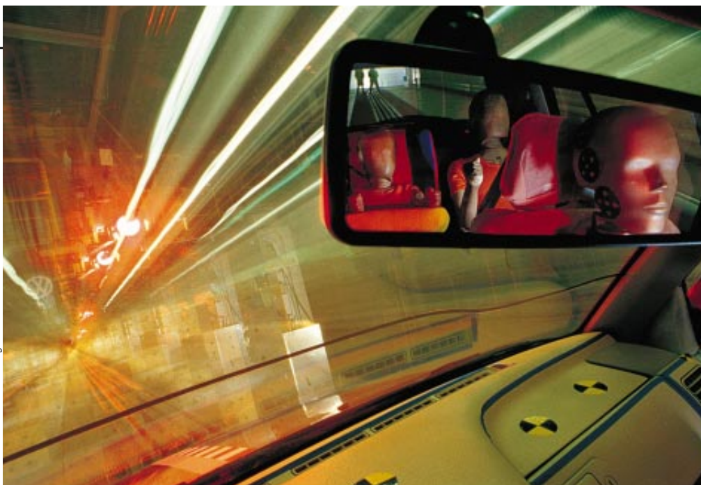
HEADING FOR A CRASH , this family of dummies is instrumented to record what happens to its members on impact. The dummies, which took their short spin at Volkswagen's safety center in Wolfsburg, Germany, cost about $65,000 apiece.
