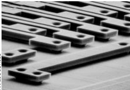
BEAMS that serve as part of an acceleration sensor for triggering air bags ( photograph ) are made by first depositing layers of silicon nitride (an insulating material) and silicon dioxide on the surface of a silicon substrate ( a ). Holes are lithographically patterned and etched into the silicon dioxide to form anchor points for the beams ( b ). A layer of polycrystalline silicon is then deposited ( c ). Lithography and etching form the pattern of the beams ( d ). Finally, the silicon dioxide is etched away to leave the freestanding beams ( e ).
