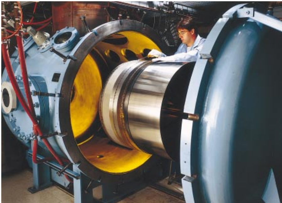
AEROSPACE COMPOSITE is manufactured in a plasma chamber at a plant owned by Textron Specialty Materials in Lowell, Mass. A worker extracts a semifinished sheet formed by spraying titanium onto a bed of silicon carbide fibers.
