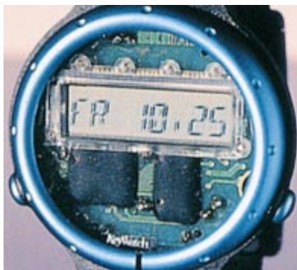
CRYPTOGRAPHIC WATCH developed by Skidata Computer in Austria contains a short-range transmitter and receiver and a microcomputer.
