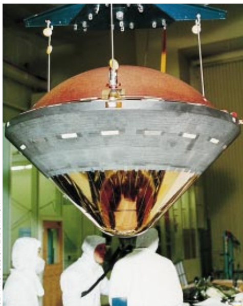
JUPITER ATMOSPHERIC PROBE will penetrate the planet on December 7. Much of the heat shield will burn away; the rest will fall off after a parachute slows the probe, exposing its instruments. These devices will measure wind speed, cloud composition, lightning frequency and other aspects of the atmosphere.
