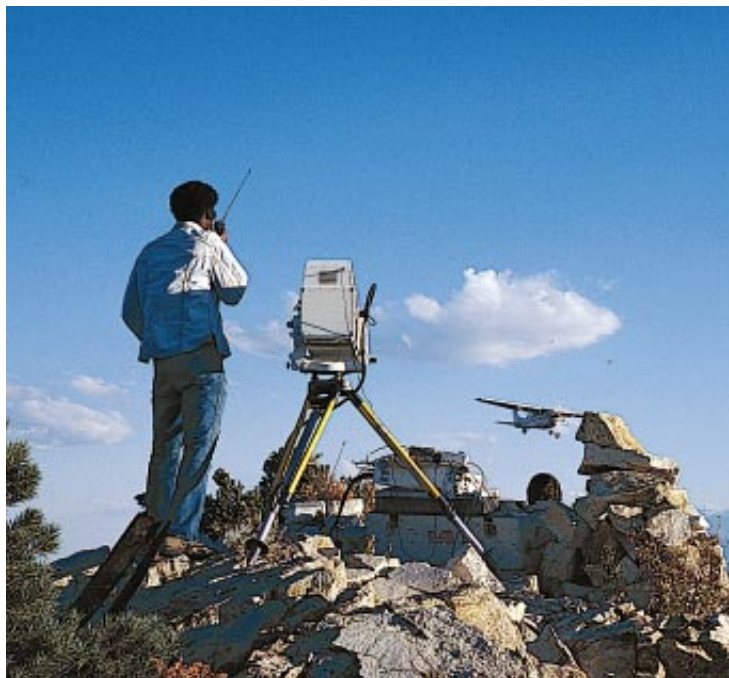
DEFORMING CRUST changes shape extremely slowly, but careful measurements can track the subtle movements of the ground. Using a laser range finder between mountaintops ( top ), scientists were able to measure horizontal contraction in the region more than a decade ago, but modern instruments that use the Global Positioning System of satellites ( left ) have eased the task of conducting precision surveys.
