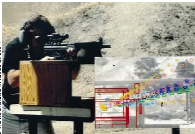
SNIPER TRACKER , developed by Lawrence Livermore National Laboratory, determines the location from which an automatic rifle ( background photograph ) fires. On the tracking screen, the cross in the rectangle at the bottom left shows the firing point. Each series of colored squares represents the track of a bullet.
