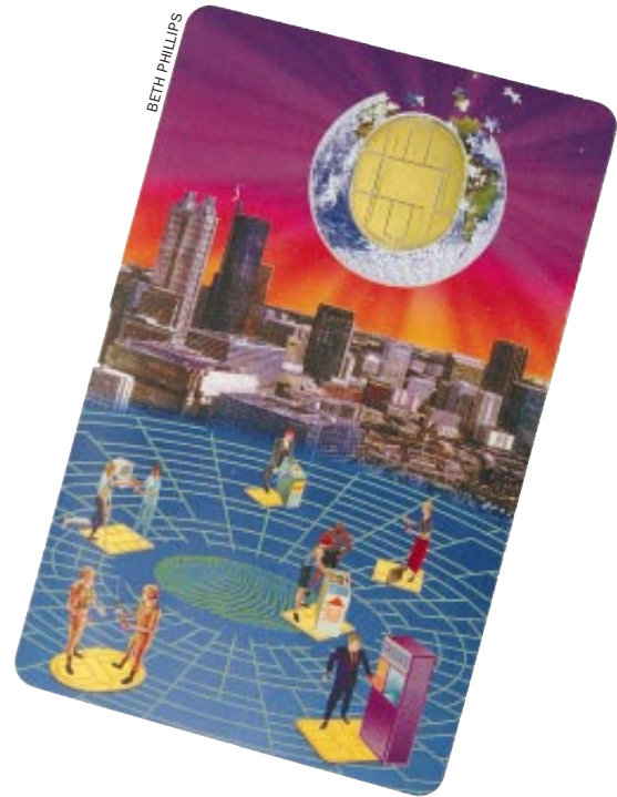
SMART CARD contains memory and a microprocessor underneath gold contact pads. The position of the pads is governed by standards so that cards and readers from many sources can work together.
