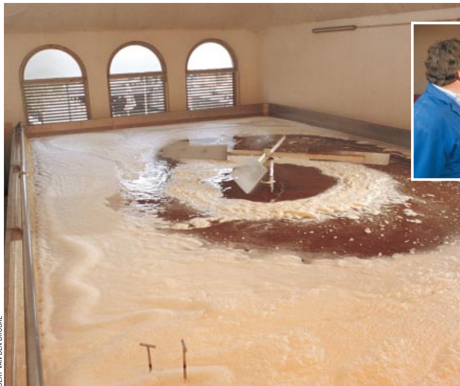
When the long boil is done, the liquid is pumped into a cooling tun in the brewery’s attic (left). This is the unique, signature event in the creation of lambic, when local microflora, including wild yeasts, inoculate the brew. Fans circulate the air while the liquid’s temperature drops to about 15 degrees Celsius (above).
