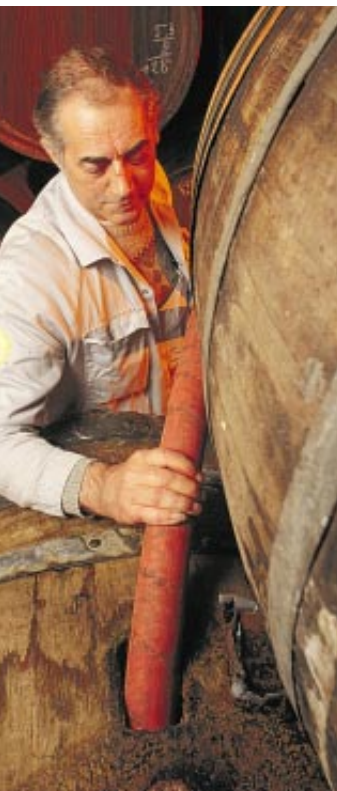
After the brew has cooled, usually overnight, it is poured into wooden casks (left) that were used previously to ferment wine. (The wood of new casks would impart an unpleasant taste.) Even after they are cleaned and fumigated, the casks contain yeast spores that help to start the fermentation. After about a week, the fermentation is so energetic that foam sputters out of escape valves in the casks (below).
