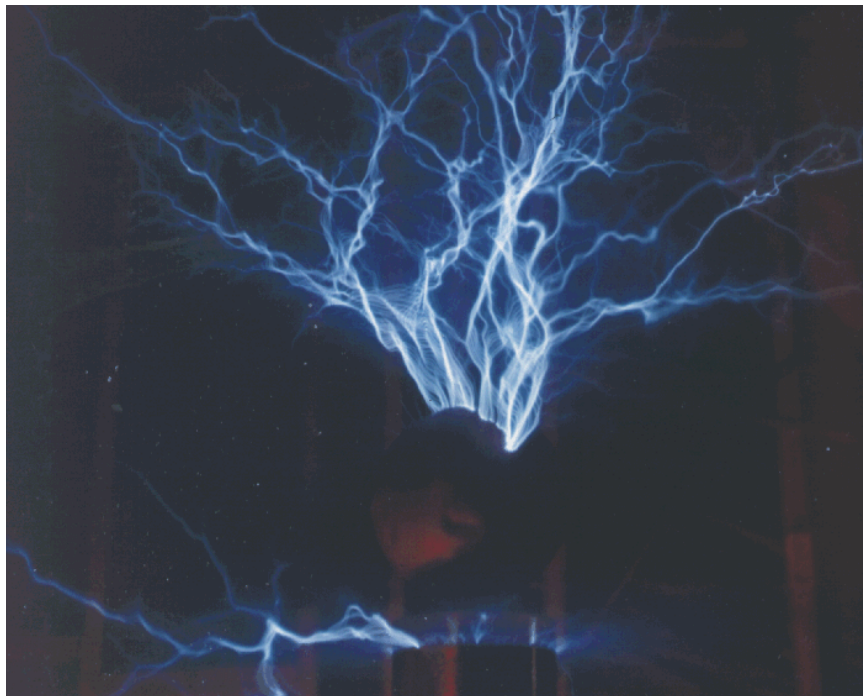
ARTIFICIAL LIGHTNING streams from the terminal of a high-frequency Tesla coil. The eccentric inventor conceived the device as part of a system that might broadcast power through the earth's atmosphere.
