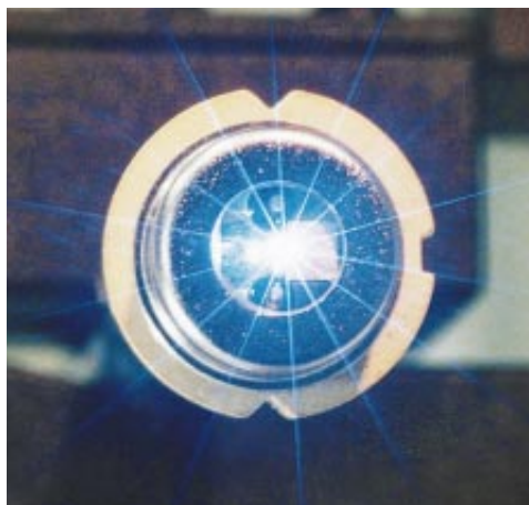
BLUE-LIGHT SEMICONDUCTOR LASER made by a Japanese researcher could revolutionize information technology.
