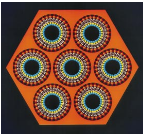
TRAP FOR HEAVY METALS, mesoporous silica is filled with channels (shown here in cross section). Each tunnel can be lined with chains bearing sulfur (yellow) to lock up mercury (blue).
