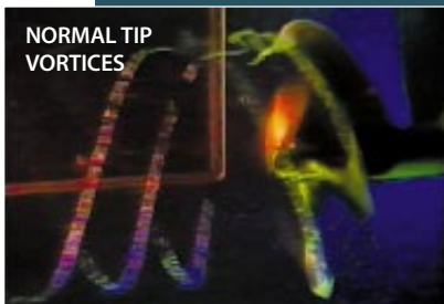
CAVITATION OCCURS ON LOW-PRESSURE SURFACE
