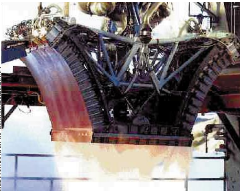
TEST FIRING of a linear aerospike engine took place at Rocketdyne's Santa Susana Field Laboratory in California during the early 1970s.
