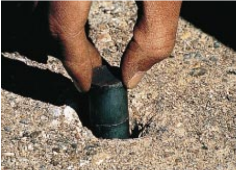
ELECTRONIC EQUIPMENT required for automated operation includes magnetometers mounted below the bumpers ( top ), magnets embedded in the road ( bottom ) and an array of other sensors, actuators and computers installed inside the vehicle ( right ).
