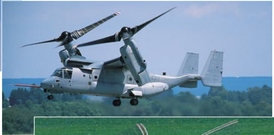
V-22 TILTROTOR can ascend vertically, with its proprotors pointing straight up. An alternative, shown here, is a short takeoff mode, which enables the craft to be more heavily loaded. In this mode the proprotors are tilted forward, providing some horizontal thrust.
