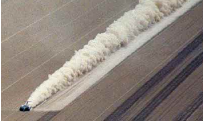
EFFECT OF SHOCK WAVE can be seen in the lateral stream of dust stretching to the side of Thrust SSC.
