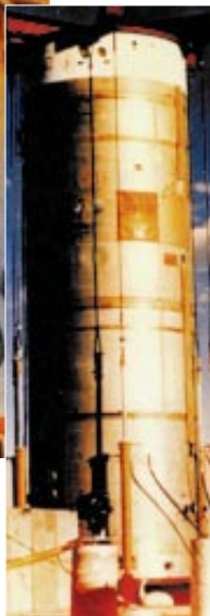
TEST OF THE MIRACL LASER was done on a Titan missile stage, which before exploding dimpled just above the halfway point, where the laser hit (inset).
