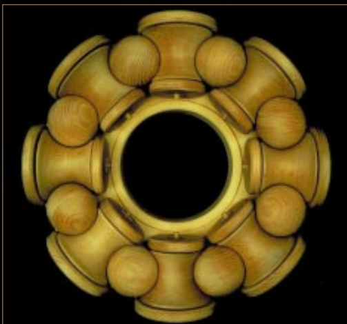
Leonardo da Vinci PRESSURE-RESISTANT BALL BEARING
