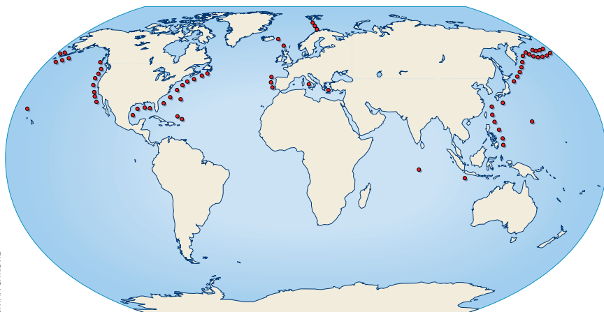
SOUND SURVEILLANCE SYSTEM, or SOSUS, consists of arrays of hydrophones deployed on the ocean floor. During the early 1980s, some 66 arrays were operating at the locations shown here; in the wake of the cold war, the number has been reduced.
