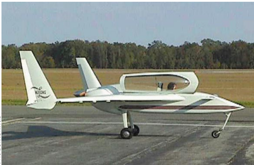
LONG-EZ is made from composites.
