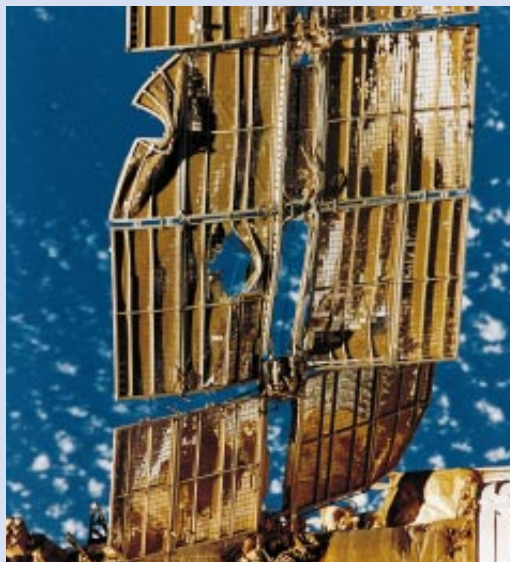
SOLAR ARRAY damaged by the Progress collision
