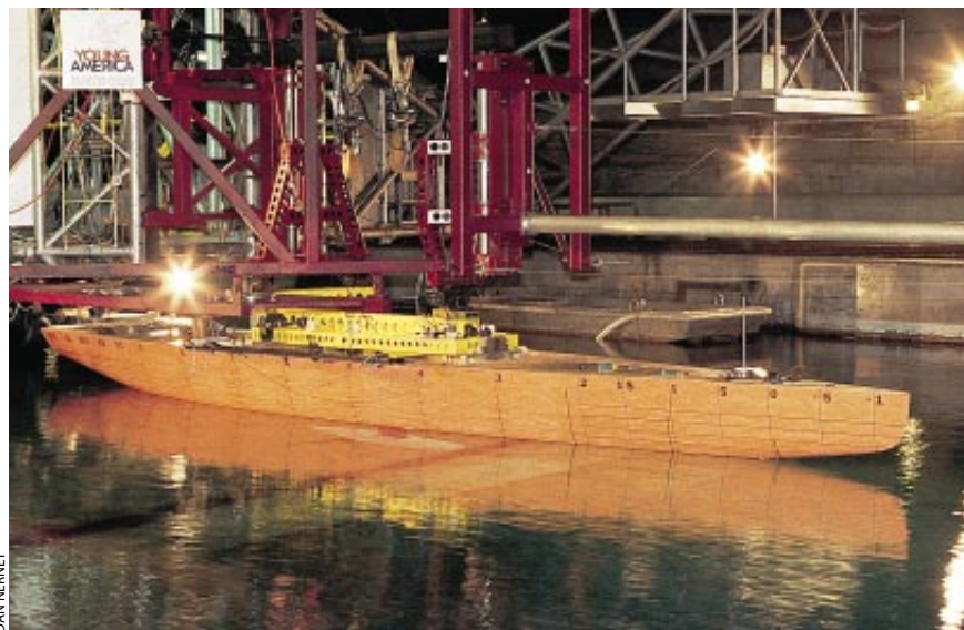
AMERICA'S CUP MODEL, measuring 7.6 meters long, sails through still waters in the testing tank at the David Taylor Model Basin in Bethesda, Md.
