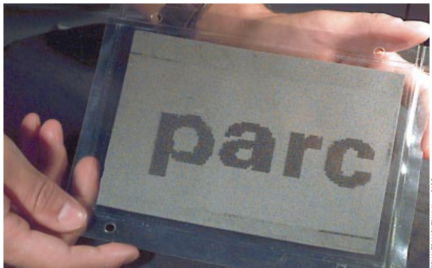
PROTOTYPE OF XEROX'S GYRICON DISPLAY, as thin as seven sheets of paper, will hold its image for months without power.
