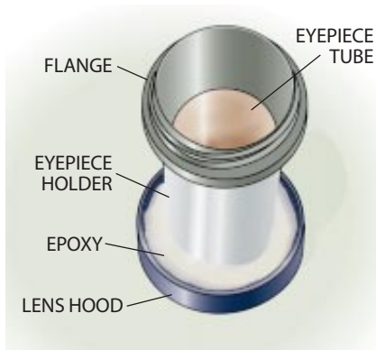
VIDEO ADAPTER is made by attaching the microscope eyepiece holder to a lens hood using quick-setting epoxy.
