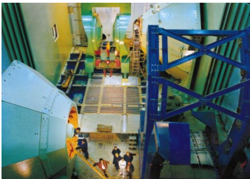
PHENIX DETECTOR , shown before assembly, includes conical “wings” designed to capture muons from a nuclear impact. Some of the steel plates in these wings, shipped from St. Petersburg, Russia, are among the largest ever cast.
