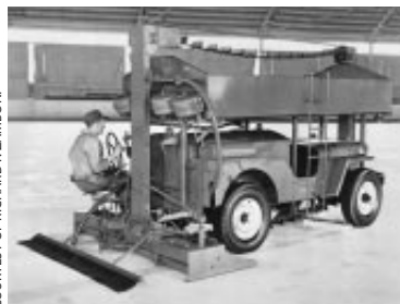
EARLY ZAMBONIS , such as this one from 1950, were built around existing jeeps or jeep chassis.
