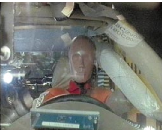
PROTOTYPE CRASH TEST was recorded by high-speed still cameras. These images, of a side-impact crash, represent the best possible visual results because they are unobscured by debris. During the collision, the head air bag deployed, keeping the dummy's head from hitting the side of the car.
