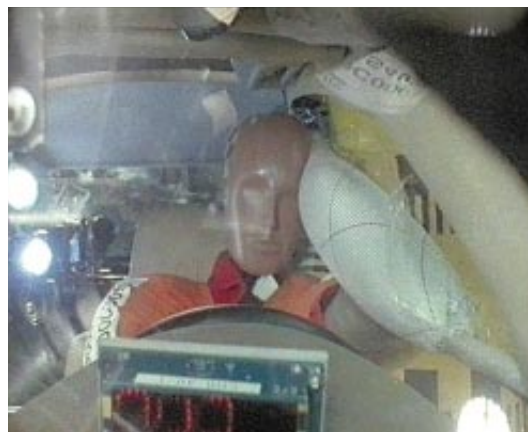
PROTOTYPE CRASH TEST was recorded by high-speed still cameras. These images, of a side-impact crash, represent the best possible visual results because they are unobscured by debris. During the collision, the head air bag deployed, keeping the dummy's head from hitting the side of the car.
