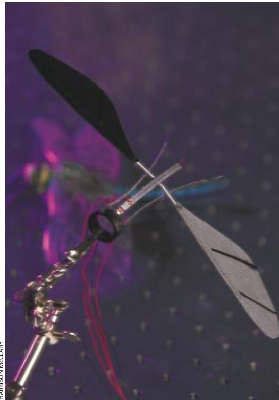
ARTIFICIAL FLAPPING INSECT built by Adam Cox and his colleagues at Vanderbilt University draws power through a tether. Such vehicles might fly freely in three years.
