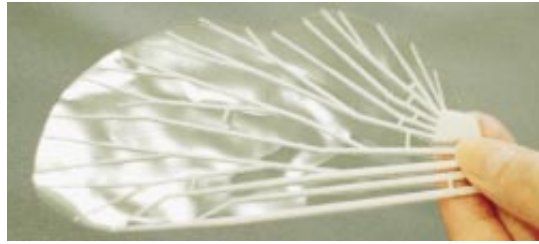
“ENTOMOPTER” WING developed at Georgia Tech benefited from work on how insects achieve lift.
