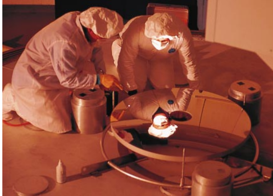
(CFHT) dome (left). In the chamber, a thin layer of aluminum evaporated on the glass disk (center). Later, Gemini's John Filhaber and CFHT coating specialist Barney Magrath, who held the flashlight, inspected the highly reflective finish (right).
