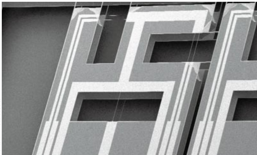
MICROSCOPIC MICROPHONE PINPOINTS SOUND in three dimensions. Thin, two-lane bridges of metal—one pair for each dimension—are heated. Passing sound waves cool one span more, creating an electrical signal.
