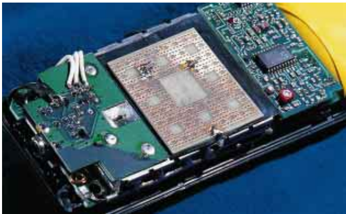
HIDDEN INSIDE a cordless phone, a square fractal antenna (center board) replaces the usual rubbery stalk.
