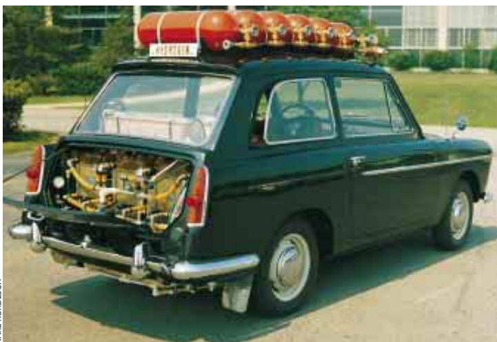
AUSTIN A40 SEDAN was equipped with Union Carbide alkaline fuel cells in 1966 by Karl Kordesch. Though historically important, the vehicle was hardly practical: the cells occupied much of the interior of the passenger compartment. Tanks of compressed hydrogen are visible on the roof.
