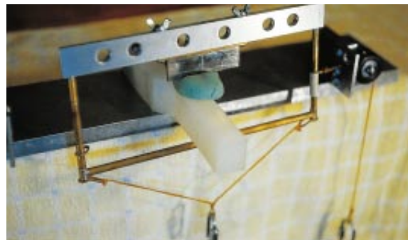
EXPERIMENTAL DEVICE (above) for measuring cutting forces of various blades: weights attached to cords at the sides and center cause the blade to make a standard cut of 10 millimeters in a meat sample (represented here by green rubber). Below is a close-up of filaments of tendon, trapped between serrations on a tyrannosaur tooth.
