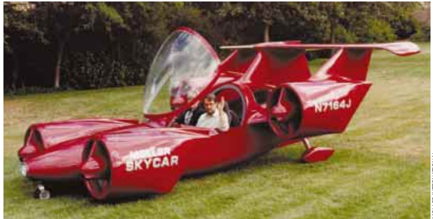
M400 SKYCAR being built by Moller International could combine vertical-takeoff capability and high speed—if safety tests planned for this winter are successful.
