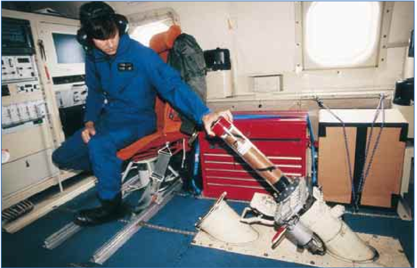
GLOBAL POSITIONING SYSTEM SONDE is readied for launch by electrical engineer Richard McNamara. Cabin air pressure blows the devices out of a floor-mounted tube. Once clear of the plane, the sondes deploy a parachute and transmit data about where winds take them during their several-minute fall to the ocean.
