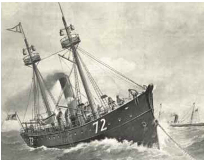
Aid to navigation: a steam-powered electric lightship
