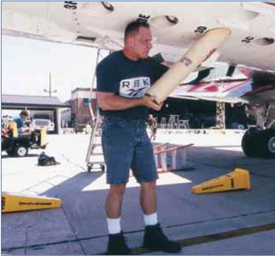
TECHNICIAN James Barr loads AXBTs into firing tubes. Explosives will shoot the probes clear of the plane during the flight.
