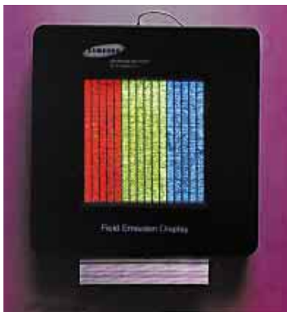
FLAT SCREEN using carbon nanotubes as the source of phosphor-exciting electrons may compete with LCDs in a few years.
