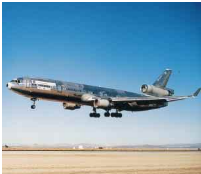
LOOK MA, NO FLAPS: Testing in 1995 showed the ability of software to land an MD-11 on engine thrust alone.
