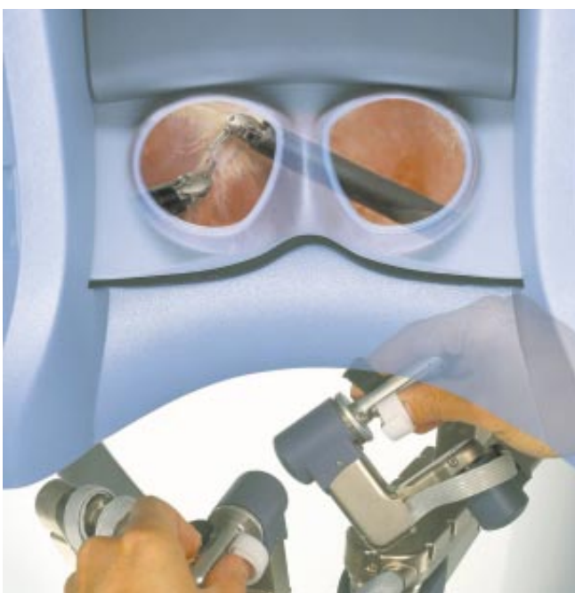
SURGEON'S-EYE VIEW during robotic heart surgery ( bottom ) reveals two tiny instruments used to perform a coronary bypass operation; additional models are shown above. Surgeons can see inside the chest cavity thanks to camera lenses inserted through a small incision between the ribs; the surgeons' hand motions at a computer console are translated to the surgical instruments.
