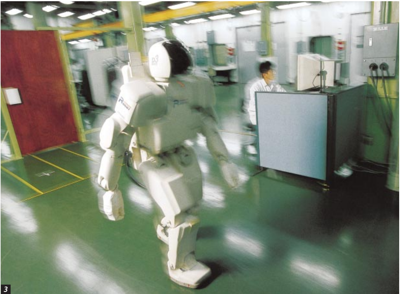
1 Researcher Cynthia Breazeal of the M.I.T. Artificial Intelligence Laboratory holds a mirror to her creation, Kismet; 2 Kismet's disassembled head reveals the mechanisms that move its features; 3 Honda P3 strides along at the company's secret research facility near Tokyo; 4 M.I.T. Leg Lab researcher Hugh Herr, himself a double amputee, is developing a robotic knee; 5 My Real Baby, a collaboration between toy company Hasbro and iRobot, can mimic the facial expressions of a human infant.
