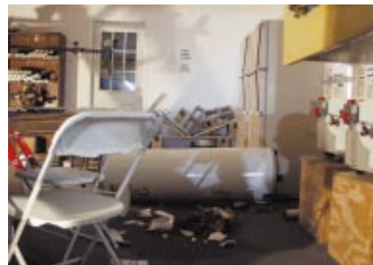
MODEL HOME (top) survived a simulated magnitude-6.7 earthquake, although the furnishings didn't fare as well (bottom).
