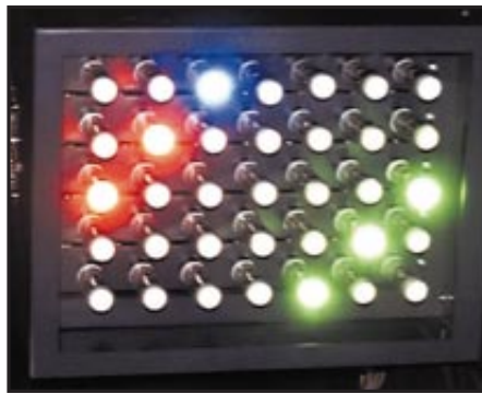
FIRST ELECTRONIC DEVICES to incorporate nanotubes include vacuum-tube lighting elements (left) and a full-color flat-panel display (right). Both products make use of nanotubes' ability to emit electrons at relatively low voltages without burning out, which translates into more efficient use of power and possibly greater durability.
