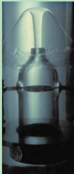
HELIUM FOUNTAIN, triggered by the heating coil, is a spectacular example of superfluidity. Up to one tenth of the helium atoms are in the form of a liquid Bose-Einstein condensate.
