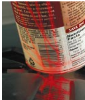
BAR-CODE SCANNING relies on semiconductor lasers.
