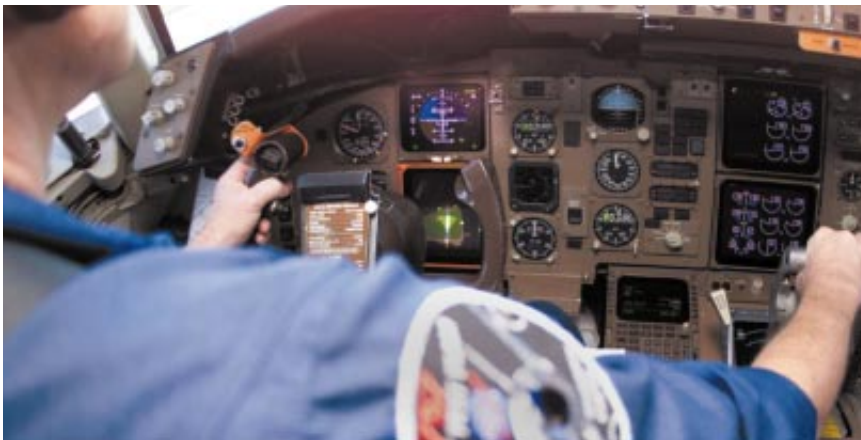
HAZARD-ALERT system by NASA warns pilots via a moving-map display (left, behind yoke and outlined by orange stripe) and a “head-up” display (above).
