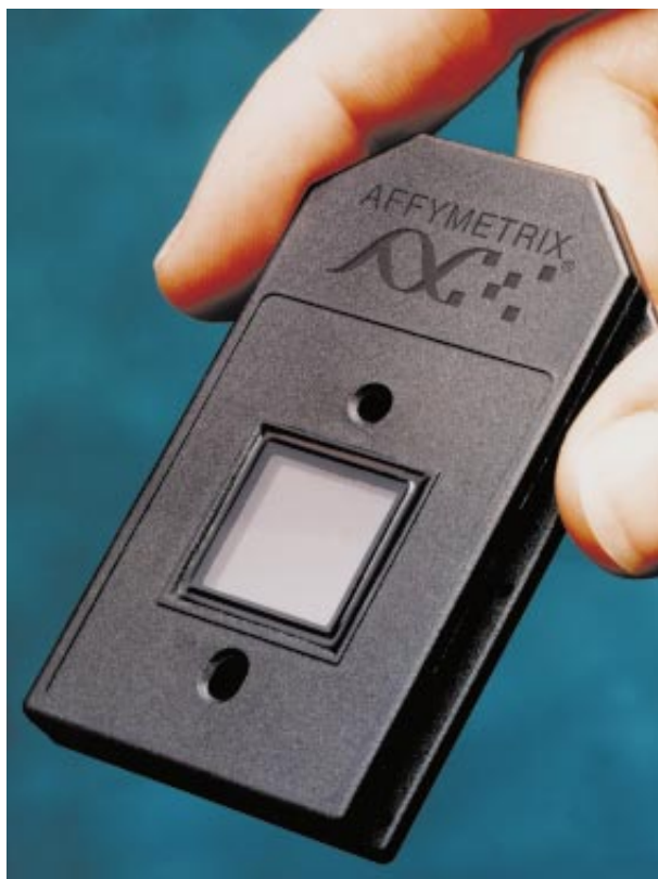
DNA CHIPS in handheld housings can sense the on/off state of up to 400,000 genes in a tissue sample.
