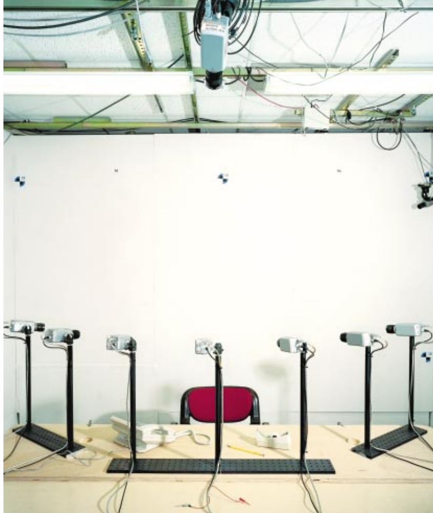
SEVEN CAMERAS scrutinize the user in the tele-immersion setup in Chapel Hill.
