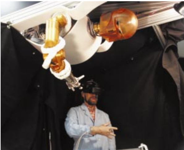
DO AS I DO: Virtual reality for controlling Robonaut's motions.
