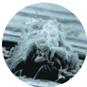
LUSH BIOFILM appeared on an industrial heat exchanger. Such contamination can reduce efficiency.
