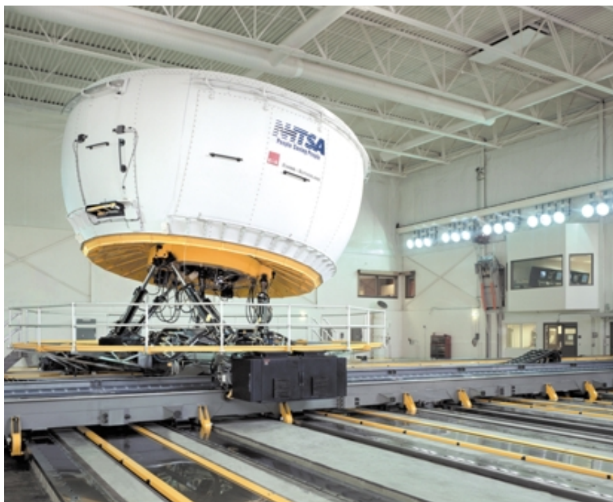
VIRTUAL TEST DRIVING of onboard automotive telematics technology is one of the functions of the National Advanced Driving Simulator [above and opposite page], which the National Highway Traffic Safety Administration recently opened at the University of Iowa.
