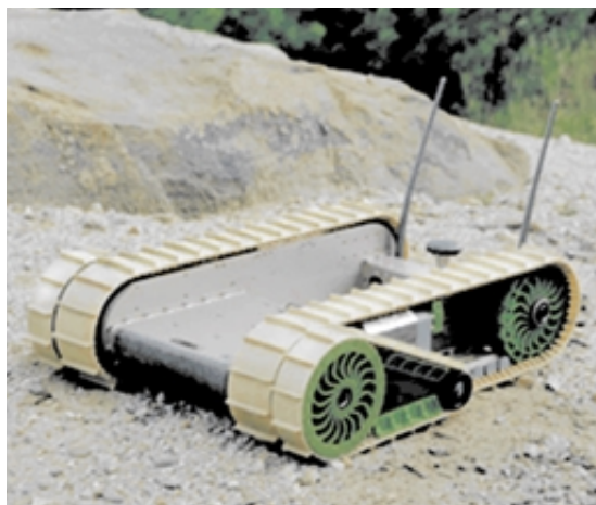
TELEPRESENCE ROBOT called the Packbot is designed to do reconnaissance in dangerous environments. iRobot, a company based in Somerville, Mass., has built other mobile machines that can transmit video over the Internet ( opposite page ).
