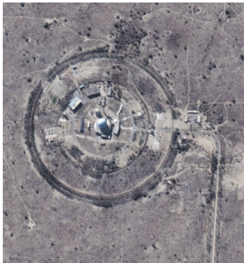
KHUSHAB NUCLEAR REACTOR in Pakistan produces a few bombs' worth of plutonium every year. Based on the size of the cooling towers visible in this Ikonos commercial satellite image, nuclear analysts estimate that the reactor generates about 50 megawatts of heat.
