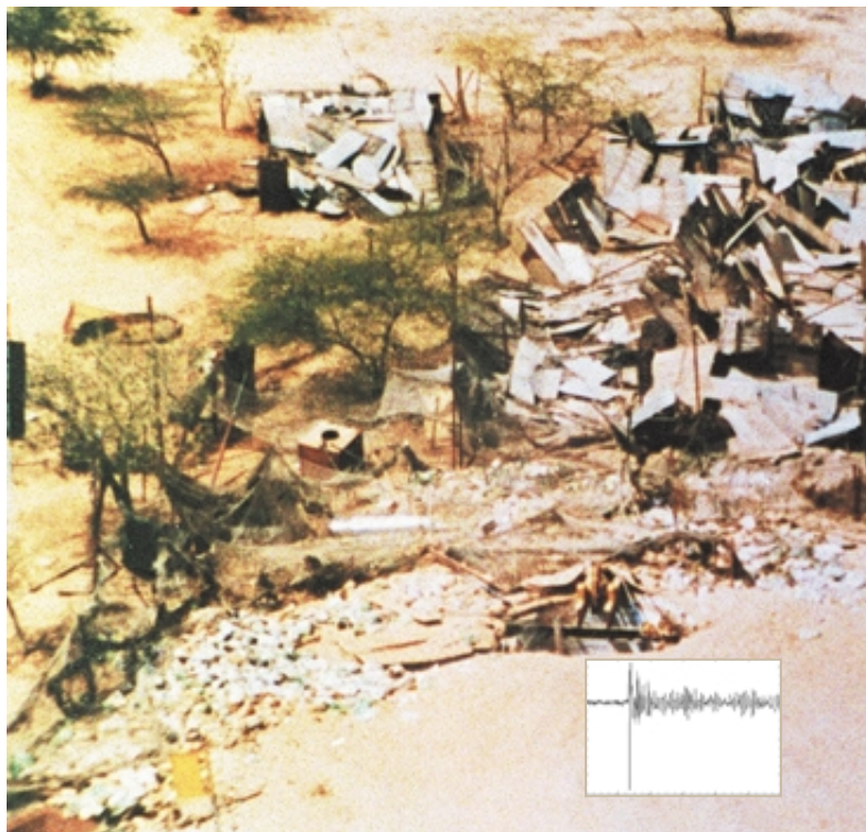
UNDERGROUND NUCLEAR EXPLOSIONS conducted by India on May 11, 1998, caused the surface immediately above to collapse. Seismic readings (inset) suggest that the total explosive yield was between 16 and 30 kilotons, about half of what India claimed.
