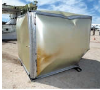
EXPLOSION causes a luggage container made from a composite material called Glare to deform without breaching.
