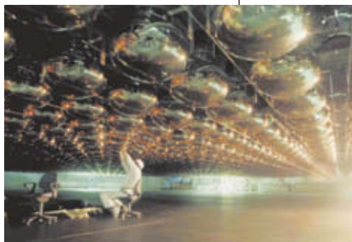
PHOTOMULTIPLIER TUBES installed in the roof of Super-Kamiokande during construction in 1995.
