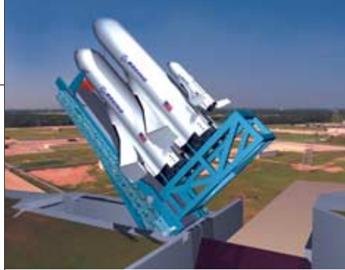
THREE-STAGE CRAFT proposed by Boeing has two large boosters that could fly back to the launch site.
