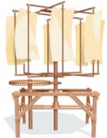
SAILS or wooden paddles of ancient windmills harnessed wind drag (push) and lift to do work, mostly to grind (mill) grain or pump water.
