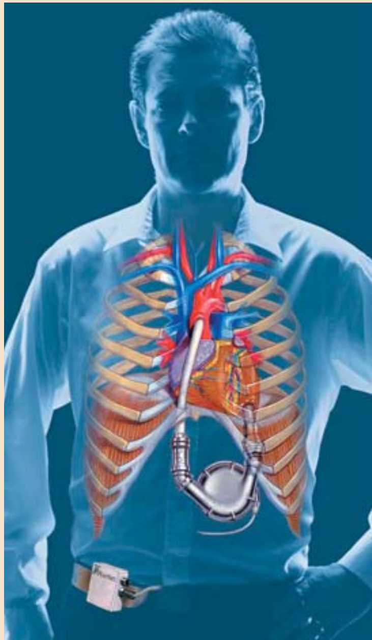
HEARTMATE PUMP, the most widely used ventricular-assist device, is implanted in a patient’s abdomen, as shown in this artist’s rendering. Attached to a failing left ventricle, the device pumps oxygenated blood to the body.
