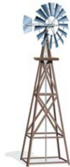
ANGLED BLADES of a farm windmill better tapped aerodynamic lift and drag to grind grain, pump water or generate electricity.
