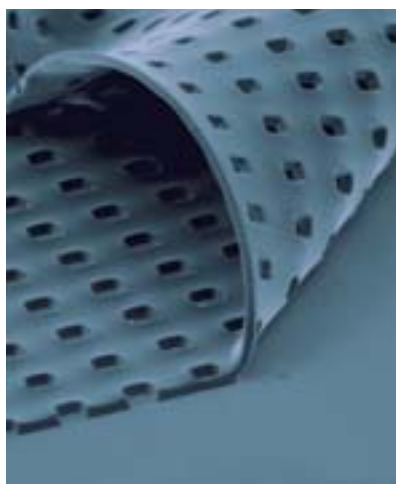
PEELING OFF a rubber sheet allows Surface Logix scientists to test how cells placed in micromolded cavities react to a drug candidate ( cells not shown ).
