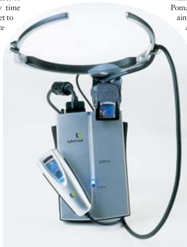
FIRST WEARABLE COMPUTER for the masses, the Poma packs a lot of power into a small package. The six-inch-high computer (center) contains a 128-megahertz RISC processor, 32 megabytes of random-access memory and an equal amount of read-only memory. The head-mounted screen (top) weighs less than three ounces. The optical mouse (lower left) allows you to move the cursor with your thumb.
