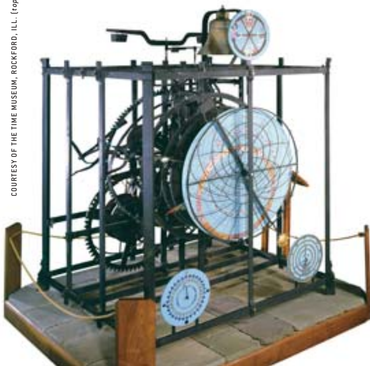
EARLY MECHANICAL CLOCK, commissioned by Richard of Wallingford, English mathematician and abbot of St. Alban's Abbey, was built between 1327 and 1336 to help his monks maintain their daily routines.
