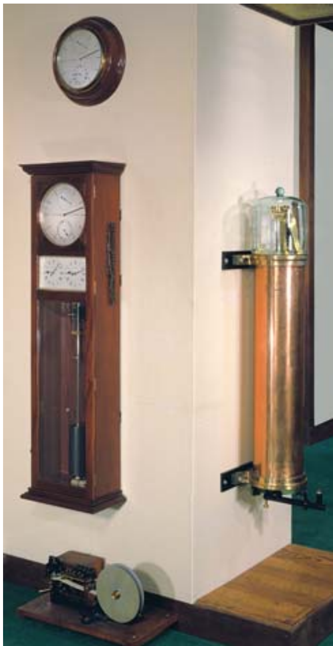
FREE PENDULUM CLOCKS were developed by William H. Shortt, an English railroad engineer in the early 1920s. Shortt's timekeeping systems, which incorporated two pendulum clocks—a "master" (right) and a "slave" (left)—were reportedly able to keep time to within about a second a year.
