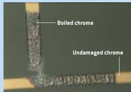
ELECTROSTATIC DAMAGE to a photomask halted production at a major European semiconductor manufacturer. The bridge defect is chrome oxide.
