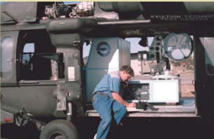
U.S. ARMY'S Long Range Biological Standoff Detection System operates on board a Black Hawk helicopter. Such lidar-based particle detectors can be coupled to biochips that can distinguish particles of harmless microbes from those containing bioweapons.
