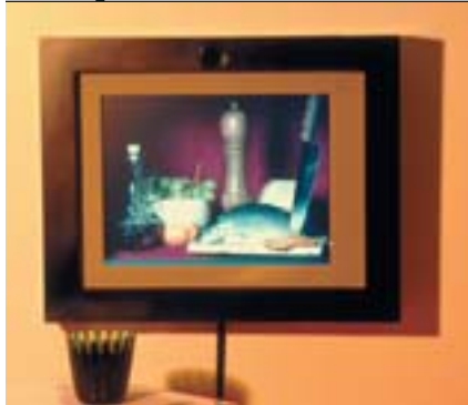
LIGHTING SENSITIVE DISPLAY developed at Columbia University changes the shadows and reflections in an image to match the exterior light. Note how the pepper mill's shadow shifts from right to left.
