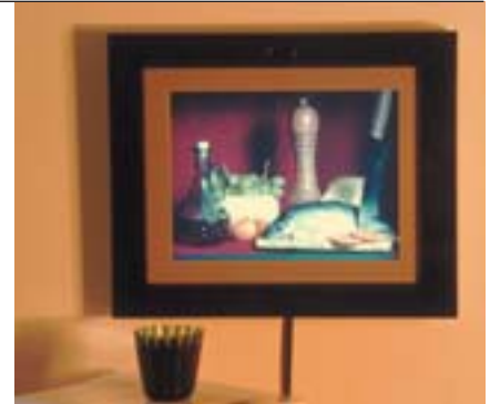
LIGHTING SENSITIVE DISPLAY developed at Columbia University changes the shadows and reflections in an image to match the exterior light. Note how the pepper mill's shadow shifts from right to left.
