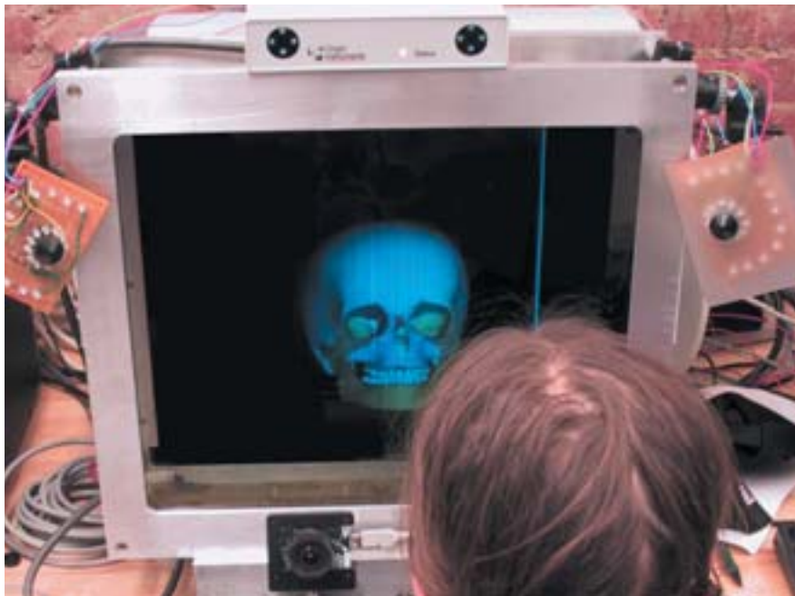
HERE'S LOOKING AT YOU: This autostereoscopic display shows a 3-D image with the help of a parallax barrier ( in front of screen ) and two infrared cameras ( on either side ) that track the user's eyes. The device was conceived at the Media Research Laboratory at New York University.
