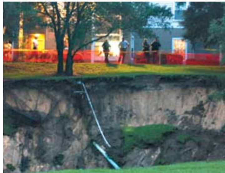
SINKHOLE , 60 feet deep and 50 feet wide, created by groundwater pumping in Orlando, Fla., June 2002.
