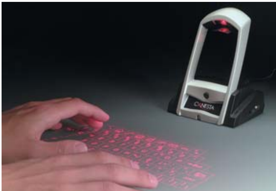
VIRTUAL KEYBOARD projected onto a tabletop allows a user of a personal electronic device to type faster and more comfortably than with input devices furnished by the manufacturer.
