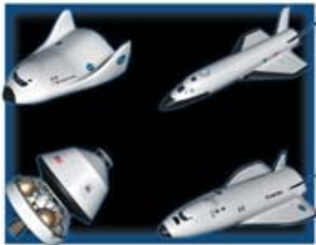
FOUR DESIGNS for the orbital space plane (clockwise from top left): lifting body; winged vehicle with sharp leading edges; shuttlelike vehicle; and capsule, which may be the safest for reentry.
