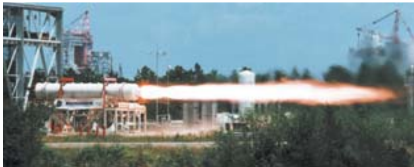
POWERFUL PLUME blasts out of a hybrid rocket motor during a ground test conducted in 1999 at NASA’s Stennis Space Center in Mississippi. An aerospace industry consortium developed the 250,000-pound thrust engine prototype as part of a $20-million program.
