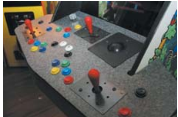
BUTTONS GALORE adorn the custom-built control panel that Aaron Mahler attached to his old Millipede game. Inside, a Dell PC serves up any of 2,000-plus arcade classics.
