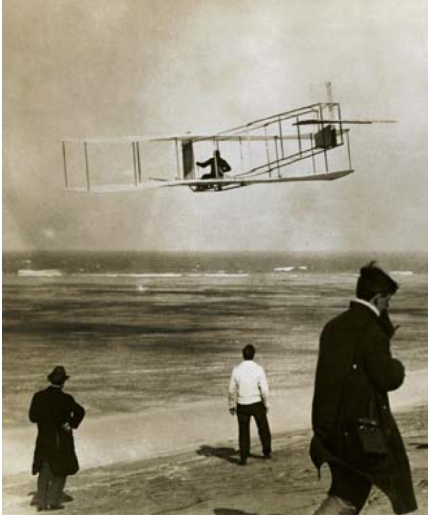
TWISTING WINGS act to create more lift on one side of this 1911 Wright brothers' glider, permitting the pilot to roll the aircraft. This pioneering wing-warping technique continued in use until elevated flight speeds necessitated stronger, more rigid wing structures.
