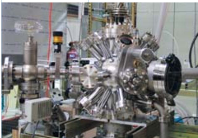
Reactor vessel uses an environmentally friendly process to clean and build microelectronic devices.
