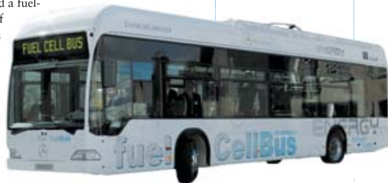
Oxygen goes in and mere water comes out of DaimlerChrysler's fuel bus.
