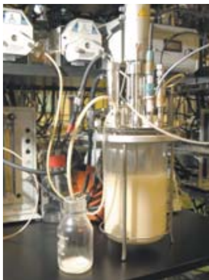
FERMENTER: A GlycoFi vessel is where protein-based drugs will be made in yeast.
