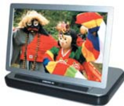
LARGE-SCREEN OLED from Samsung SDI Company measures 15.5 inches diagonally—but is only 1.8 millimeters thick.
