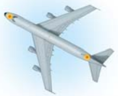
FLIGHT DATA RECORDER (in tail) far exceeds an automotive black box. It stores the last 25 hours of aircraft altitude, direction of flight, speed, acceleration and thrust from each engine. A cockpit voice recorder (in nose) captures 30 to 120 minutes of crew conversation and ambient sounds. The units can withstand impact at 268 knots, fire of 1,100 degrees Celsius and pressure of 20,000 feet undersea for 30 days.
